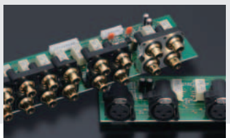
Gold-plated input/output jacks connected directly to relays
